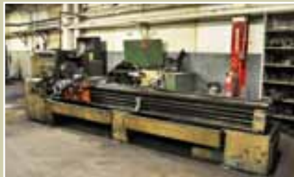
LEBLOND MDL. 1610 HEAVY DUTY SERVO SHIFT GEARED HEAD ENGINE LATHE, S/N: 2NB-692
