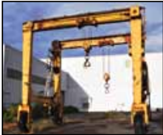
DROTT MDL 500 30 TON CAPACITY MOBILE TRAVEL CRANE SYSTEM, S/N: 2249 AXP/10100552
